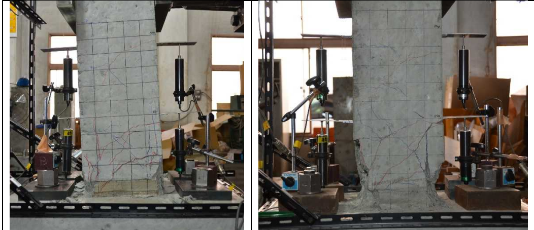
Figure 4 Crack propagation of RRC columns
