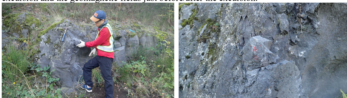
Fig. 1. Sampling at a lava flow of Volvic volcano in Massif Central (left photograph). Rock samples were oriented by using the three-point orientation tool with a magnetic compass (right photograph).
