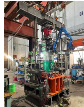
(b) FRP repaired RC columns under strong earthquakes
