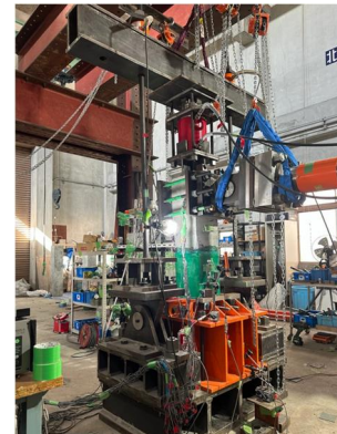
(b) RC columns under strong earthquakes
