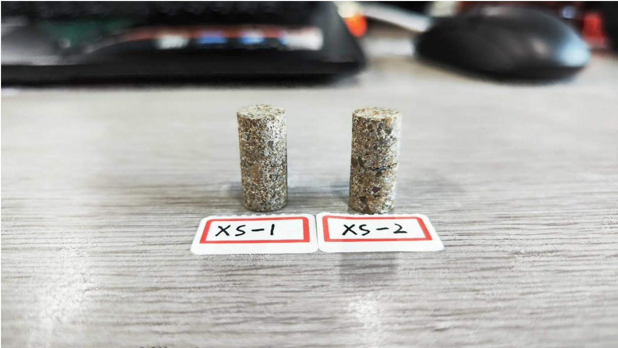
Figure 1: Sandstone specimens with a discontinuity
