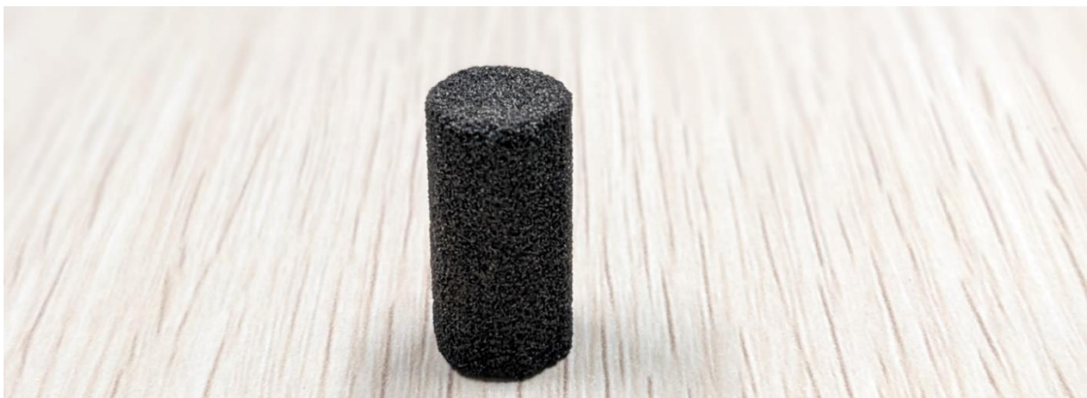
Figure 1: 3D printed specimen with a diameter of 10 mm and height of 20 mm
