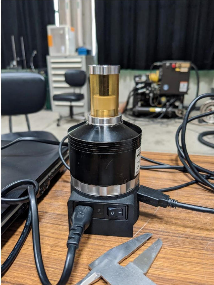
Figure 2: Small-scale uniaxial compressive test
