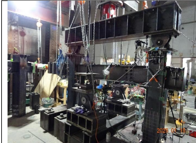
Photo 1 Experiment of CFST column with steel beam
