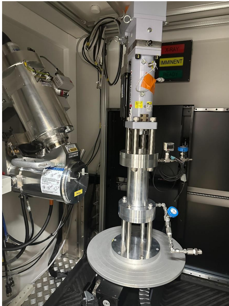
Figure 1: Newly developed triaxial testing machine for the micro-focused X-ray CT scanner
