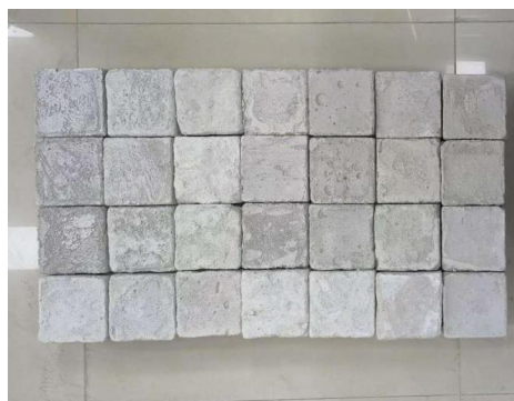
Figure 2. Cured Specimens of Alkali-Activated Fly Ash-Slag Foamed Concrete
